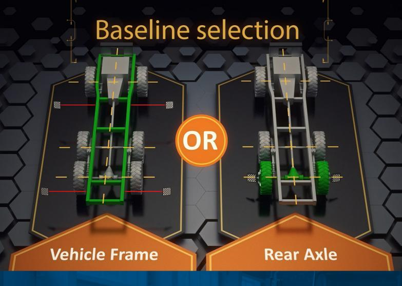
Two adjustment baselines are supported: references to the frame or vehicle centerline.
